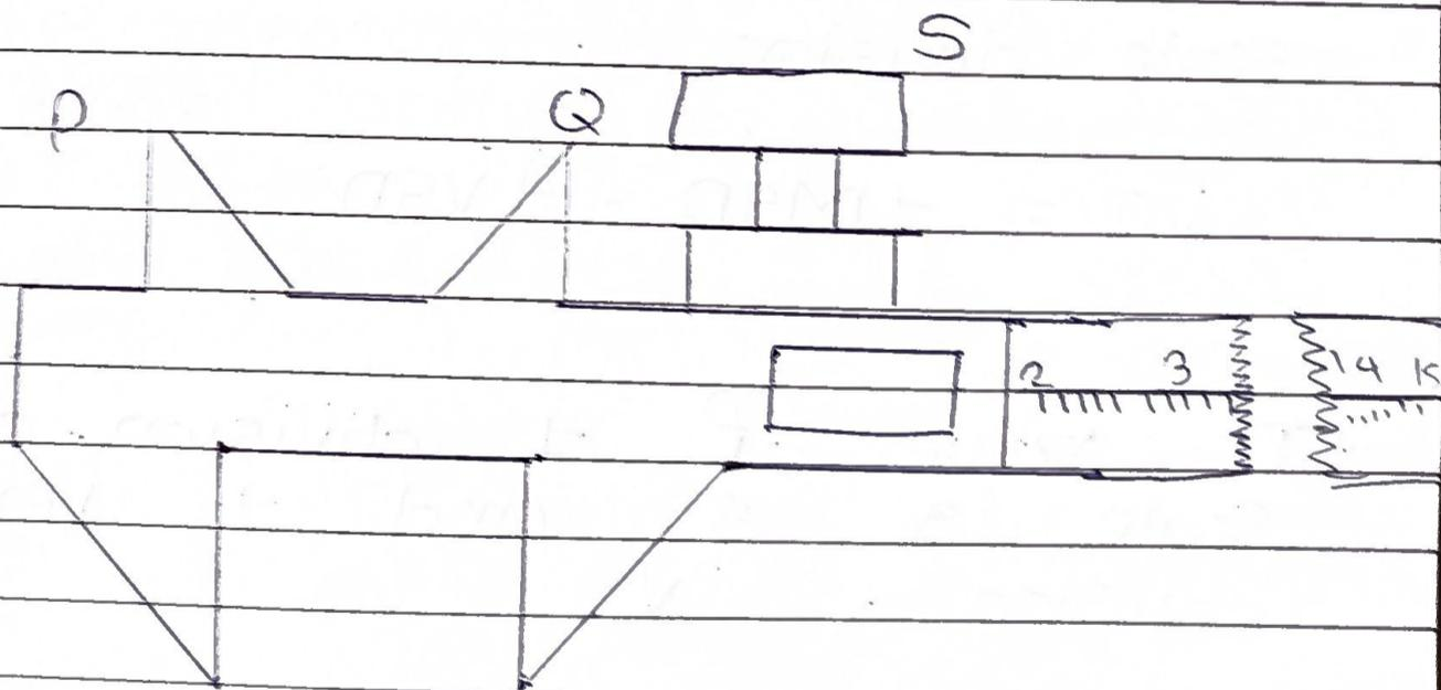
It is an instrument to measure up to smaller length up to  $\frac{1}{10}$  mm accurately
