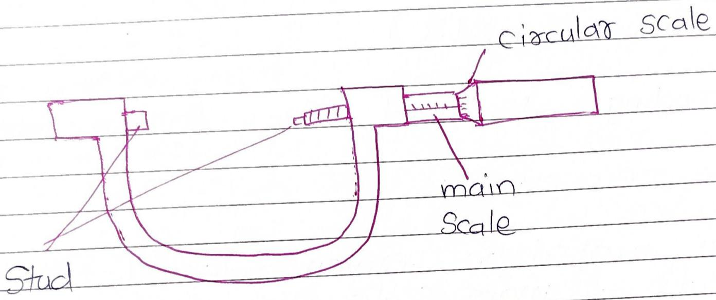
Screw gauge consists U-shaped metal frame
